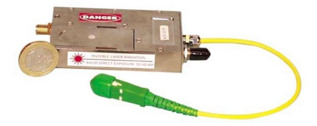
The MELOPEE **T 2001** system is designed to optically transmit an analog signal within the **5 kHz** to **5 GHz** frequency range. It consists of a compact battery powered **modem-sensor**, a 100 m long **fiber optic** cable and a broad bandwidth remote **receiver unit**. The T2001 system can transmit low level voltages, for example the output signals from **passive sensors** such as THALES E-3602.
